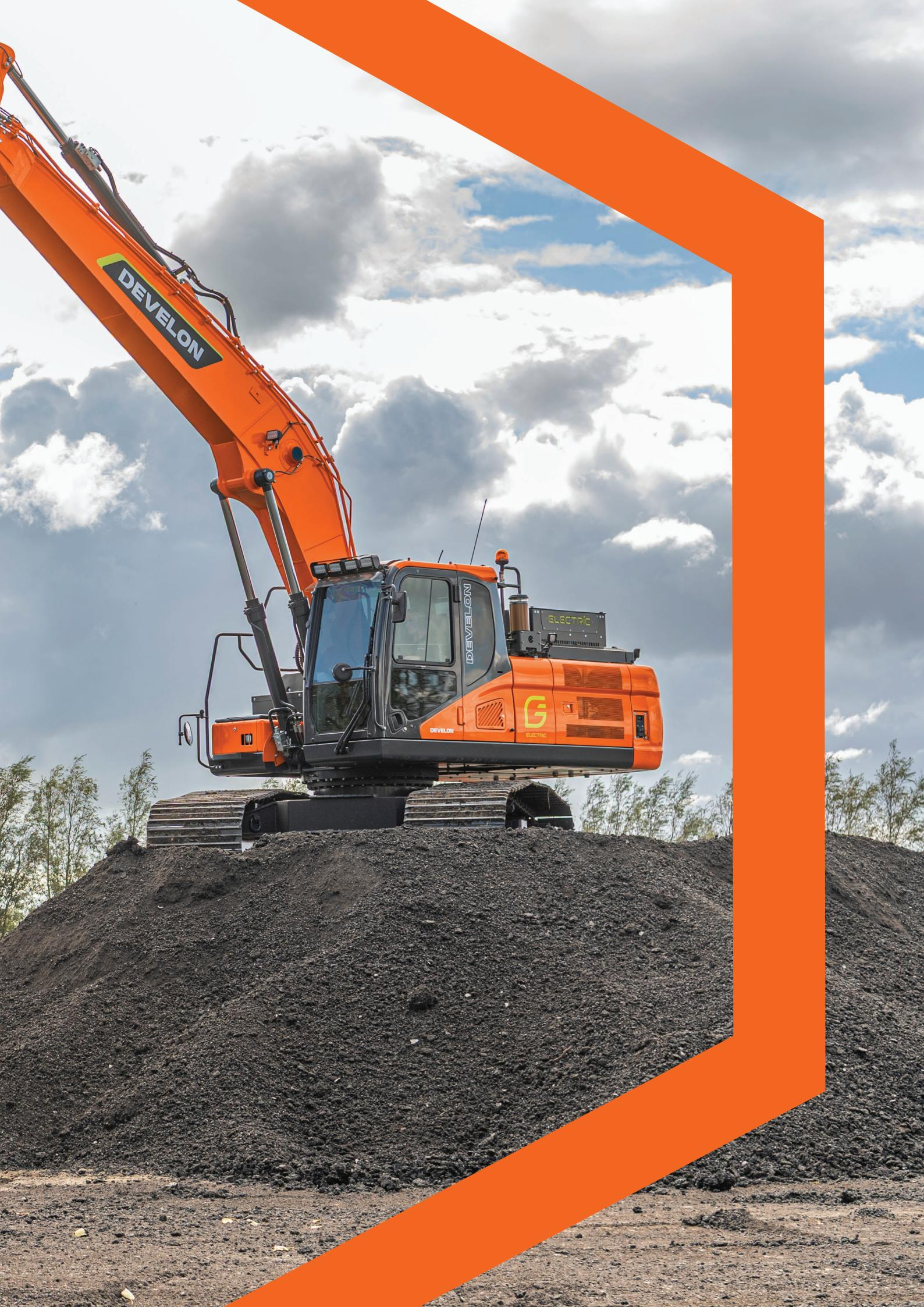
With a 120 kW liquid-cooled permanent-magnet motor, high-capacity LFP battery, and strong hydraulics, the DX230LCE-7 and DX250LCE-7 match comparable diesel crawler excavators – only quieter and emission-free at the point of use – so you can work where diesel is restricted, keep noise low on urban sites, and still get the responsiveness, force, and attachment capability your business demands.
