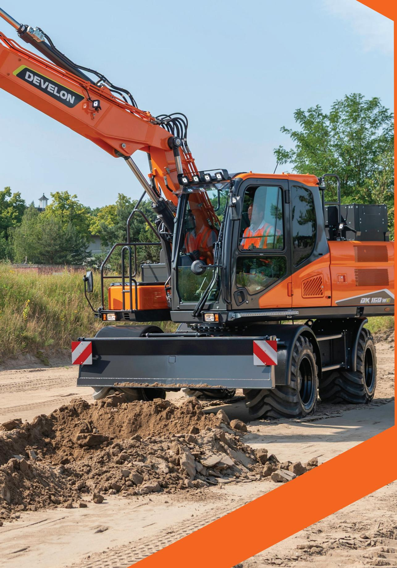
Our electric wheel excavators combine a high performance with a powerful LFP battery with full-day runtime, top-class hydraulics, and smooth, precise operation. The motor and battery deliver consistent torque, while fine swing and the Load Isolation System enhance control and operator comfort. Flexible charging options minimize downtime, helping the machine handle demanding tasks efficiently and accurately – making it a reliable, high-performing electric solution for any job site.
