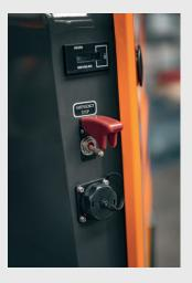
The strategically positioned emergency cut-off button provides instantaneous disruption of all machine functions, swiftly halting operations in critical situations.
