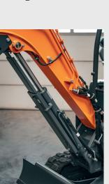
Arm, boon bucket cylinder protections engineered to withstand the challenging job site environments, ensuring longevity and durability for your equipment.
