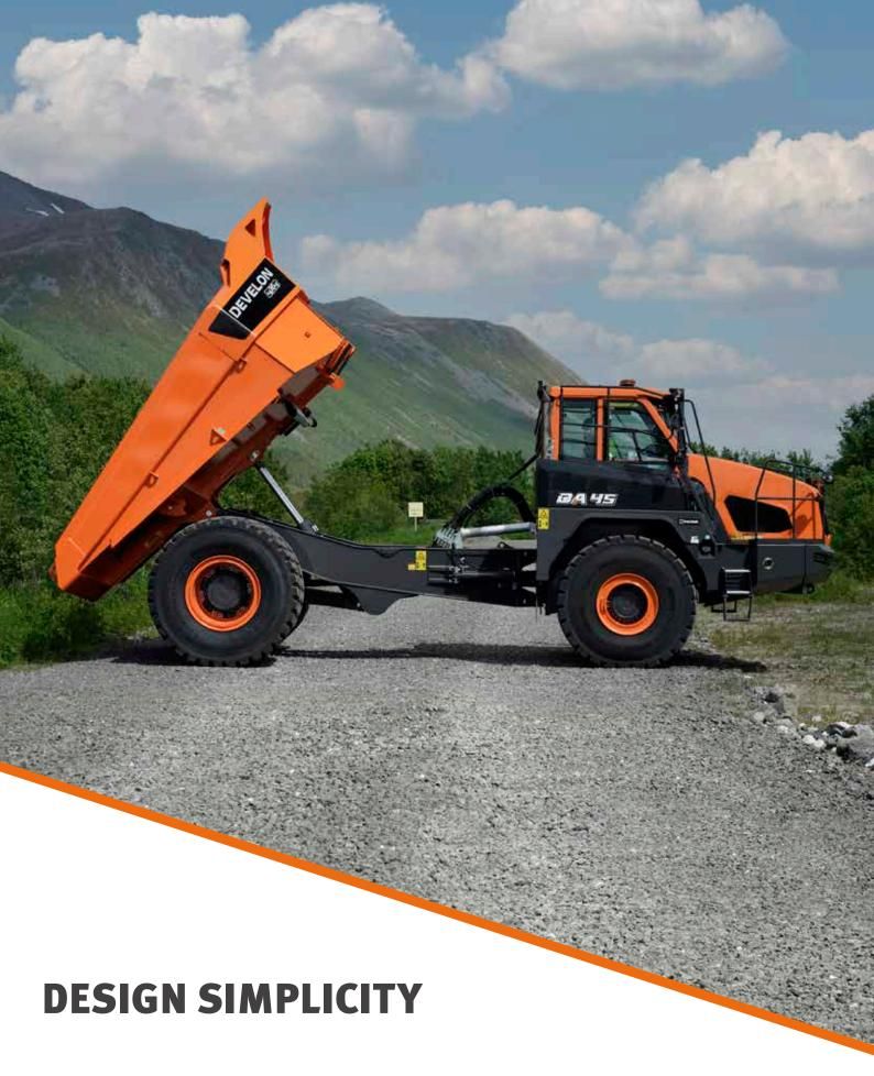
Our special front-mounted turning ring provides equal power & weight distribution and excellent operating performance. The sloping rear frame provides a lower center of gravity — improving the ADT's overall stability and ensuring fast and easy tipping of the body for increased productivity.
